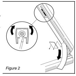
Turn the collar two or three complete turns. Then, release the brake and see if the control head moves. Continue adjusting in increments of two or three turns as needed.
