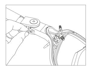
**5** Back out the 2 set screws on the side of the knuckle that retain both the top and bottom snubbing pins.
