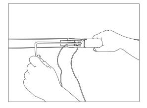
**9** Remove the 4 Flat head screws on the bottom side of the flex arm.
