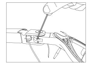
Unscrew the bottom and top snubbing pins. Be sure to hold light head during removal.
