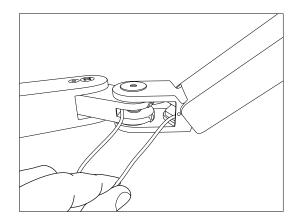
Relieve tension on backside of the flex arm with the Pelton & Crane Spring Tool, DCI PN 8697.
