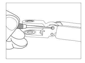
Once the pin is out, the front knuckle can be removed.
