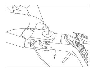
**7** Pull out the wiring from the back side of the flex arm. Do not remove the wires from the transformer side.
