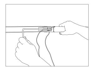
**20** Pull the arm to the horizontal position. Once the tension screw lines up with the drilled hole insert a 9/64 hex wrench to adjust drag.
